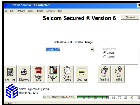
Main Screen w/standard Unit Selected Showing Command Buttons and Menu's available after Site
