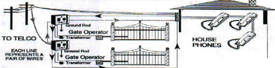
RESIDENCE WITH MULTI-LINE CONFIGURATION W/PBX SG-1 on its own TELCO line.
