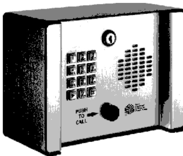
**A Wiegand digital output is available. Entering digits (can be 1 to 5 digits programmable), will send 26 bit Wiegand signals to any card reader input device capable of reading Wiegand 26 bit signals.**
